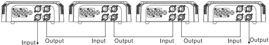
The number of daisy-chained fixtures is limited by the number of DMX channels required by the fixtures in relation to the maximum 512 channels available in one DMX universe. Note that if independent control of a fixture is required, it must have its own DMX channels. Fixtures that are required to behave identically can share the same DMX address and channels. To add more fixtures or groups of fixtures when the above limit is reached, add a DMX universe and another daisy-chained link.
