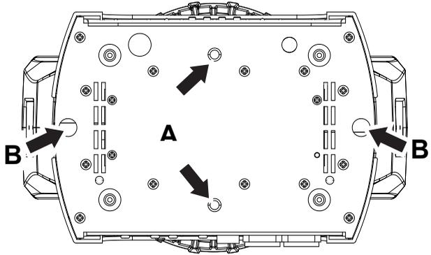
5. Working from a stable platform, hang the fixture on the truss (see illustration below) and fasten the rigging clamp onto the truss so that the fixture is suspended securely.
