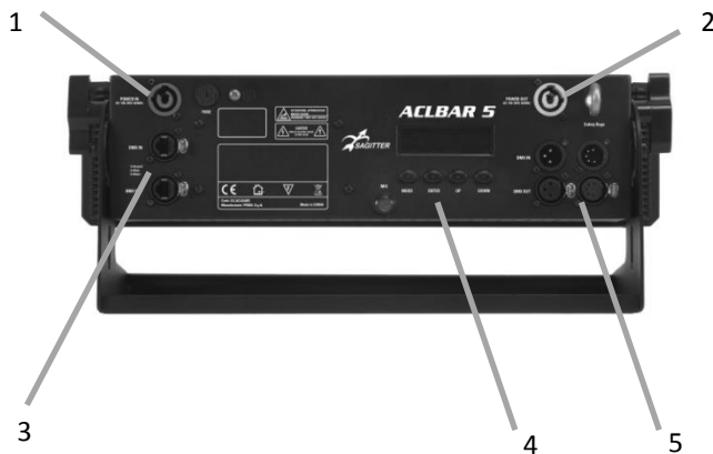
REAR VIEW 1 – Power IN 2 – Power OUT 3 – Artnet IN/OUT 4 – Display + keypad 5 – DMX IN/OUT
