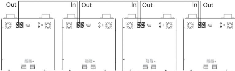
The number of daisy-chained fixtures is limited by the number of DMX channels required by the fixtures in relation to the maximum 512 channels available in one DMX universe. Note that if independent control of a fixture is required, it must have its own DMX channels. Fixtures that are required to behave identically can share the same DMX address and channels. To add more fixtures or groups of fixtures when the above limit is reached, add a DMX universe and another daisy-chained link.
